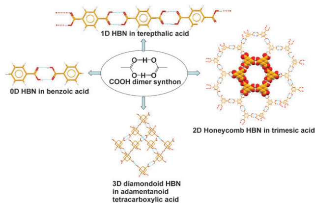
Scheme 3 Illustration of the COOH dimer supramolecular synthon and its application in crystal engineering.
