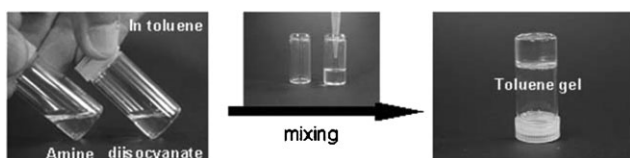
Scheme 1 Typical procedure of in situ gelation. Reproduced from ref. 20 with permission. Copyright 2004, Royal Society of Chemistry.
